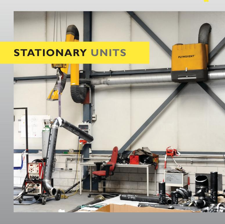
Effective welding fume extraction with stationary units SFD and SFS
